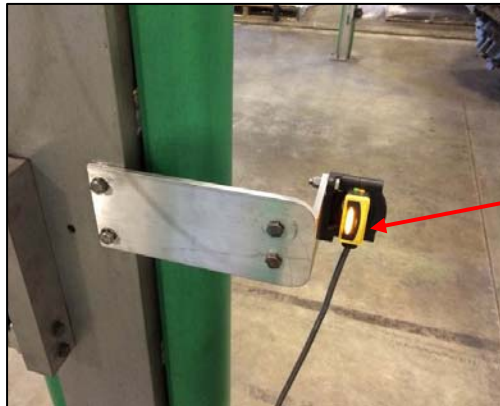
Pic #15: Photo-eye Light ON
