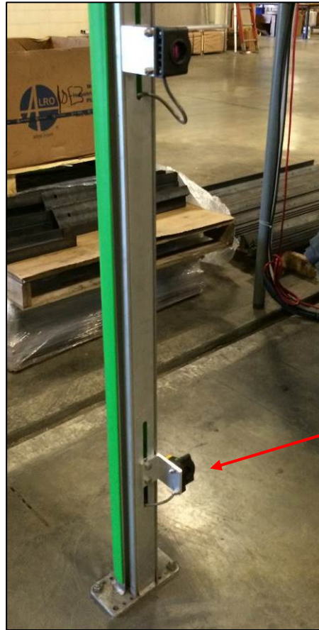
Pic #6: Emitter Photo-Eye Mounted
