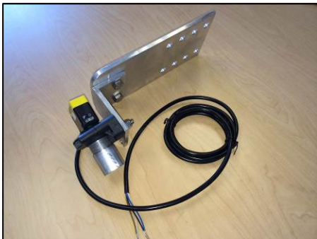
Pic #1: Receiver Photo-Eye Assy
