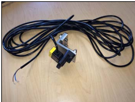
Pic #2: Emitter Photo-Eye Assy
