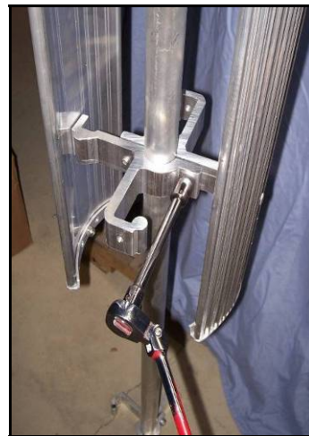
Pic #14: Adjust Core Height
