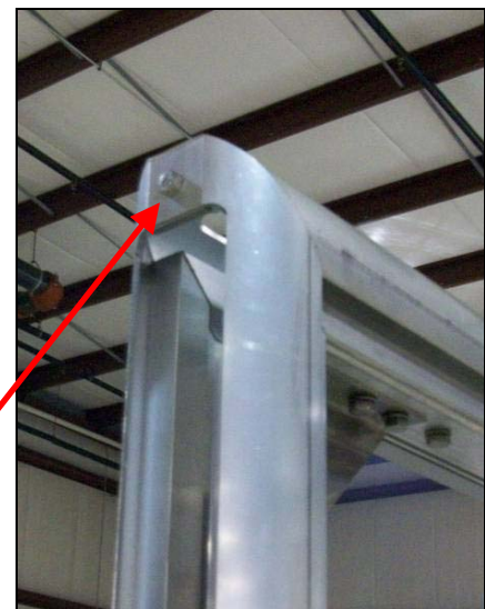
Pic #6: Secure Outside Corner to Leg Assembly
