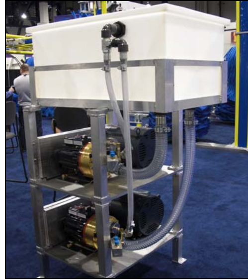
Pic #2: Dual 15HP Pumping Station
