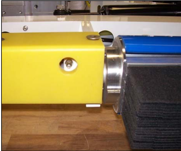
Pic #29: Entrance End Brush Bearing (1 Fitting)
