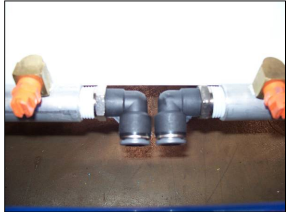
Picture #9 Manifold Fittings
