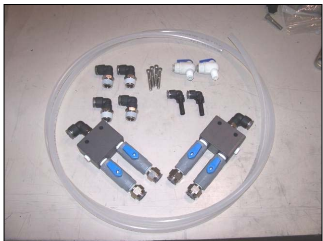
Picture #2: Tubing and "Y" Fittings
